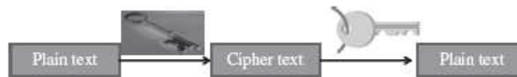
Fig: Public key cryptography (uses two keys—one for encryption and other for decryption)
